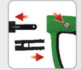
Press the Button to Pull the Metal Tube (Easy access to spare blade storage)
