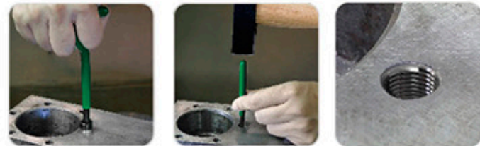
4. Screw coil into casting 5. Using pin breaking tool, break off pin on insert 6. Thread is repaired and ready to use
