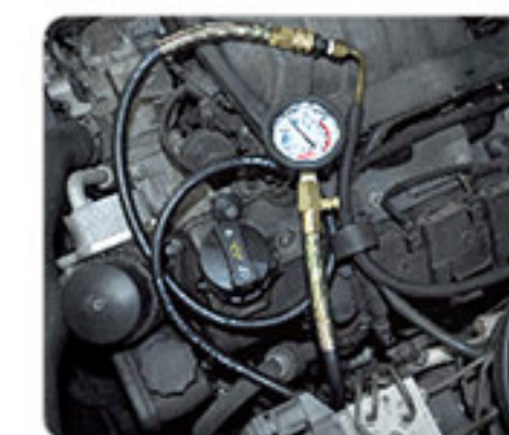
2-1/2" Diameter Gauge (150 PSI / 10 BAR) with Relief Valve, 51" Hose with Quick Coupler
